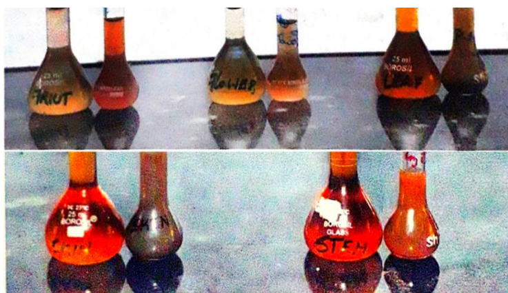
Figure 1. Color change of Punica granatum extract with \text{AgNO}_3
